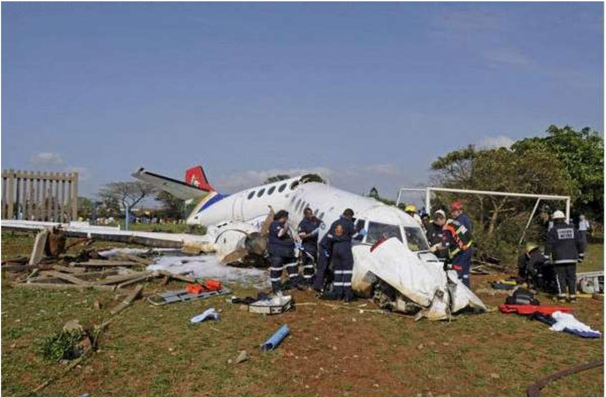
The aircraft crash landed following engine failure at take off and crashed into a concrete paling fence, see left hand side of the top photograph.
